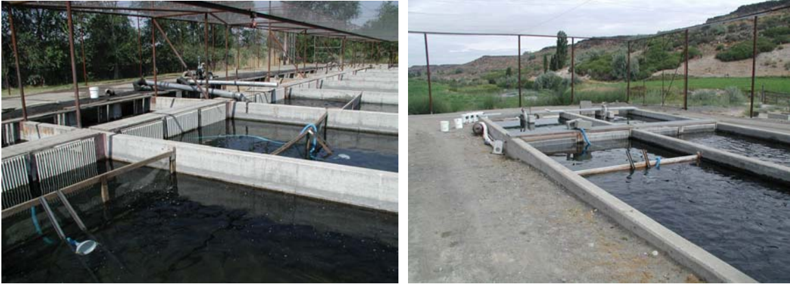
Figure 9. Funnel and siphon system used to sample influent q-zone water during q-zone size testing. Left shows q-zones 1.5 and 2 times the current length and right shows 1.5 current q-zone length.
