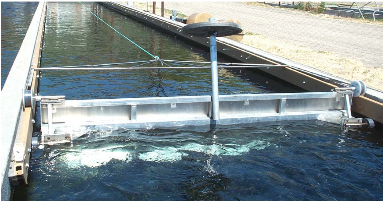
Figure 37. Second generation moving baffle prototype during commercial scale field testing in Southern Idaho.
